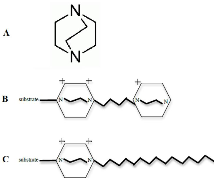
**Figure 3. Different types of DABCO-conjugated molecules.** (A) The basic structure of a DABCO molecule. (B) diDABCO-C4 molecule consisting of two DABCO molecules connected by a hydrocarbon chain of four carbons. (C) DABCO-C16 molecule consisting of a DABCO molecule with a hydrocarbon chain of 16 carbons.
